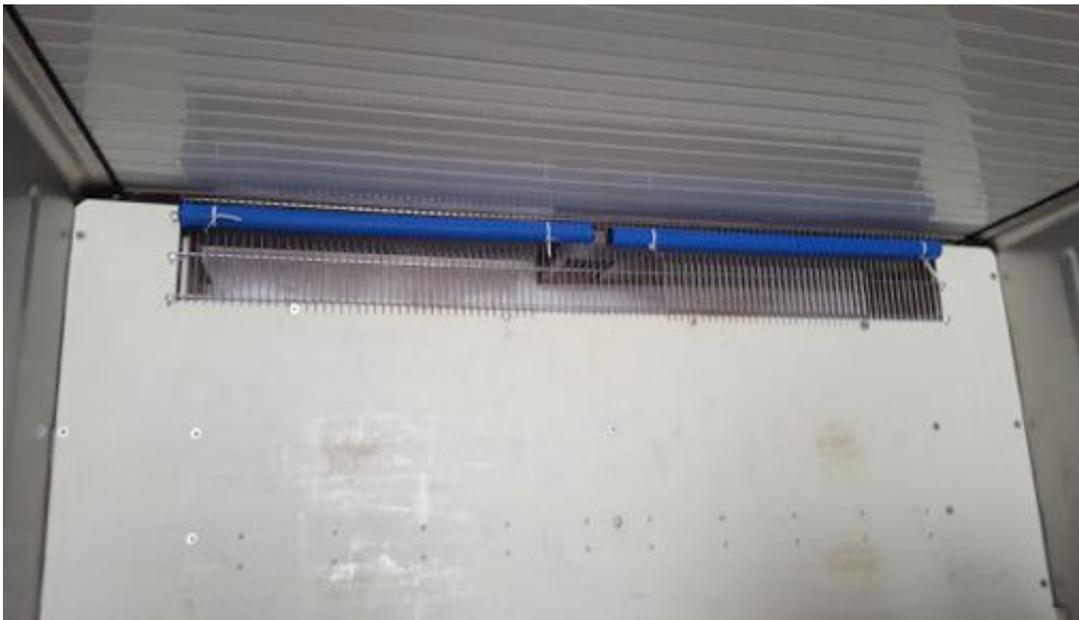
**IMPORTANT: Cold equipment must be turned off while filters are installed with flanges in the grid of the cold equipment and must be turned on after the fruit is loaded and the container door is completely closed**
