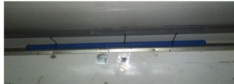
**IMPORTANT: Cold equipment must be turned off while filters are installed with flanges in the grid of the cold equipment and must be turned on after the fruit is loaded and the container door is completely closed**
